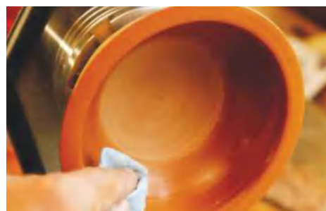
▲ Apply the Treatex with the lathe running on a slow speed and burnish as it runs
